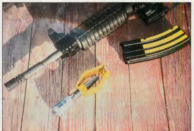
Shown for the first time is the HKM4's unique blank-firing device for use in training.
