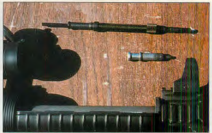
After removal of the top handguard, the gas-piston/operating rod takes seconds to remove for cleaning.
